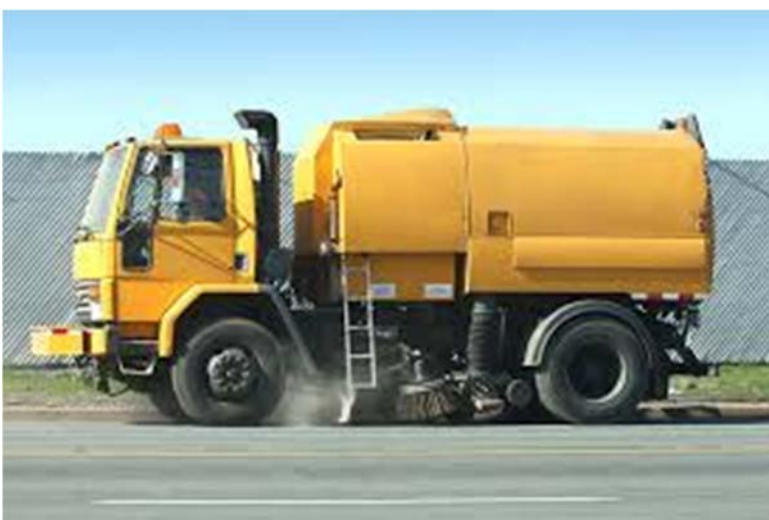
Figure 6.4 – Typical Road Sweeper
